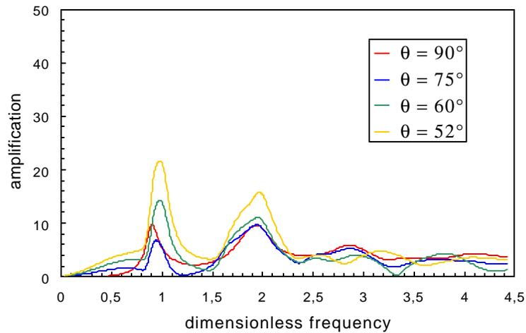
Figure 7: Response at dam crest to SV wave excitation. Empty reservoir.
