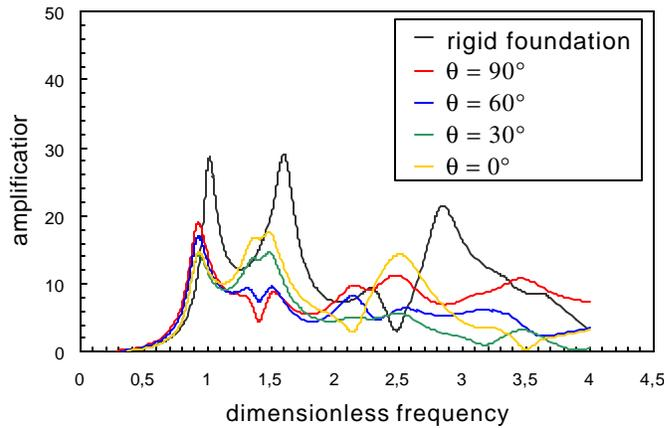
Figure 3: Response at dam crest to SH wave excitation. Empty reservoir.
