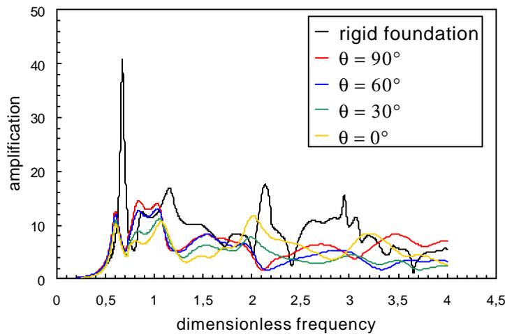
Figure 4: Response at dam crest to SH wave excitation. Full reservoir.
