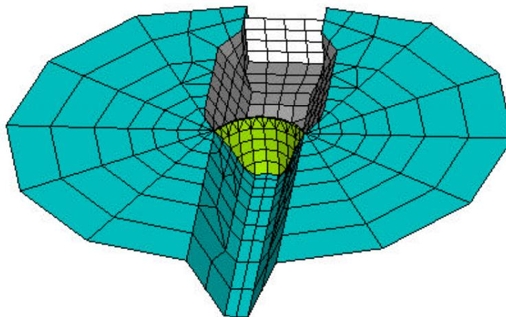
Figure 2: Boundary Element discretization of Morrow Point dam on compliant foundation rock.
