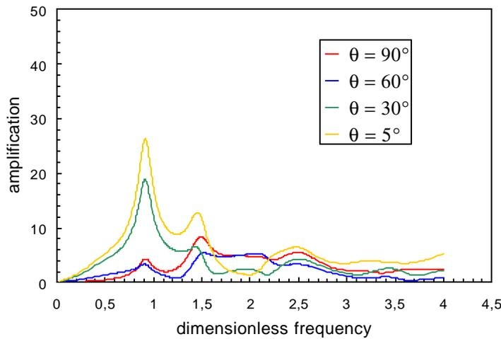
Figure 5: Response at dam crest to P wave excitation. Empty reservoir.
