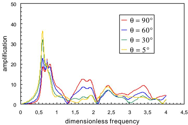
Figure 6: Response at dam crest to P wave excitation. Full reservoir.
