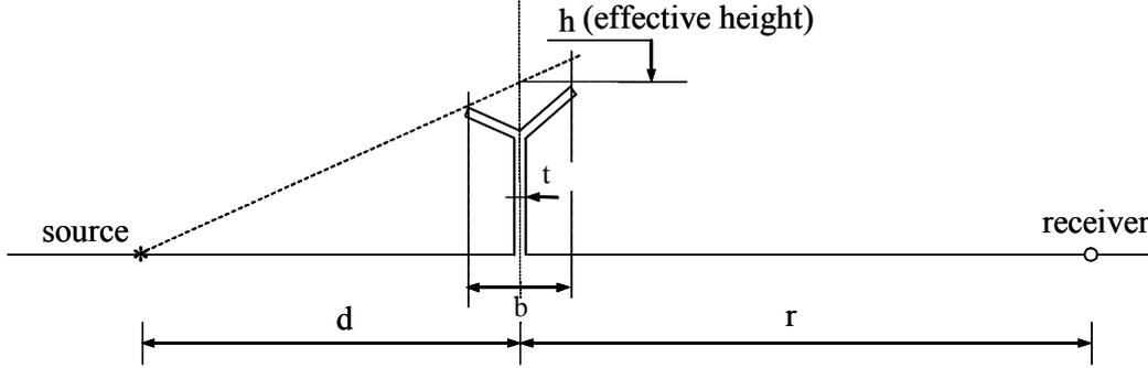
Figure 1. Two-dimensional configuration studied. Generic geometry of a three-arm barrier. All boundaries are perfectly reflecting.
