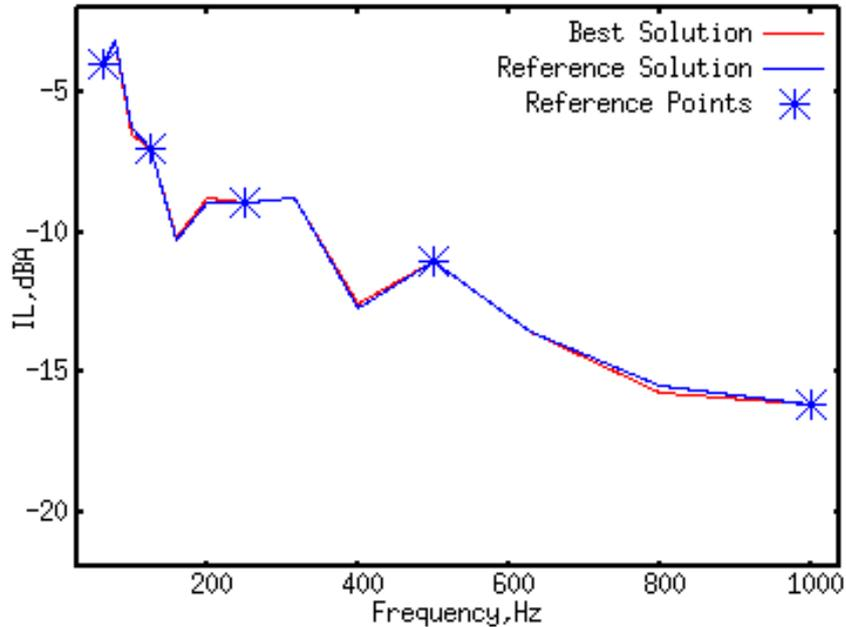
Figure 5: Comparison of IL curves of Reference Solution and Best optimized Solution (one-third octave band in graphic representation).
