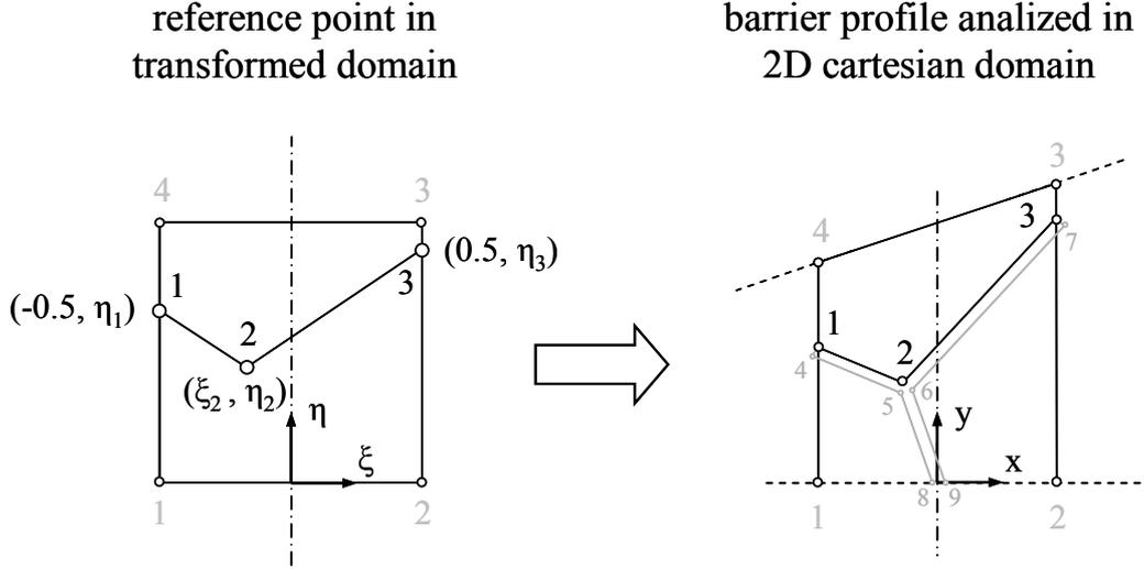
Figure 3. Process to obtain the 3 arms-profile barrier.
