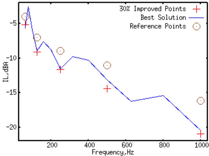
Figure 7: Comparison of IL curves of Reference Points, 30% improved Points and 30% Improved Best Solution (one-third octave band in graphic representation).
