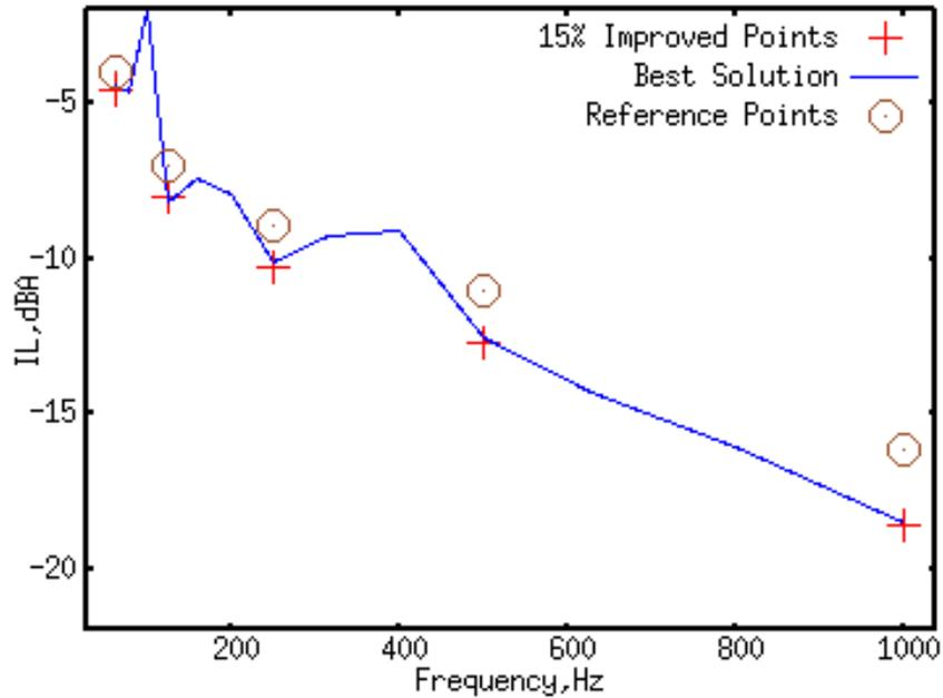
Figure 6: Comparison of IL curves of Reference Points, 15% improved Points and 15% Improved Best Solution (one-third octave band in graphic representation).
