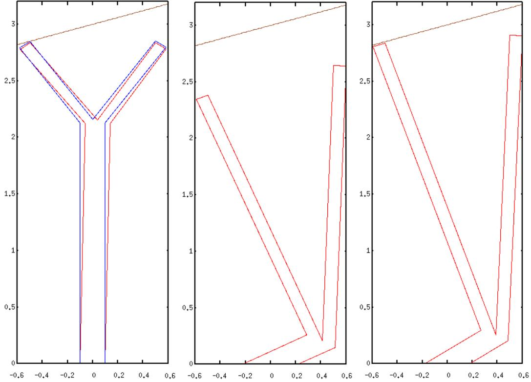
Figure 4: Sound Barriers Shapes corresponding to the solutions: inverse (left), 15% improved (middle) and 30% improved (right), in red; and initial reference, in blue.
